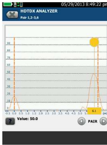
High Definition Time Domain Cross talk (HTDXT) shows the far end connection is clearly the issue
